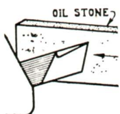
Fig. 10. Oil stone for honing cutting edge of cutter bit.
